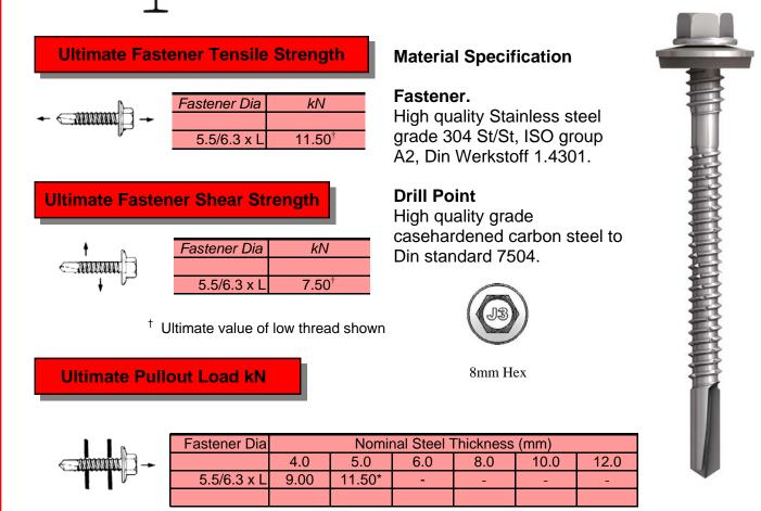
\* Ultimate pullout from steel 6.0 mm or thicker is restricted by tensile strength of fastener
